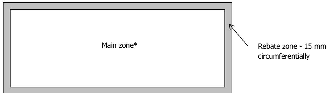
\* - If information, that glass edges are visible, is placed in order - the rebate zone is omitted and the main zone extends to the edge of the pane.
